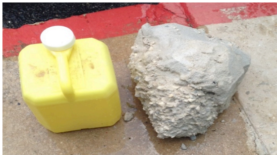
Non-compliant filter media causing high TDH
