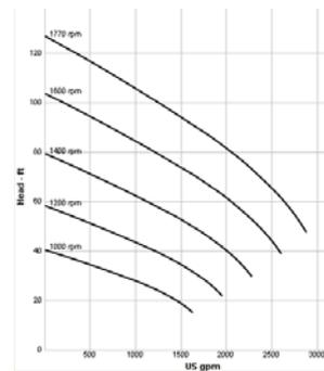
lower speeds. To answer these questions, we turn to the affinity laws. Below are the three most common equations used to predict pump performance when the impeller diameter held constant.
