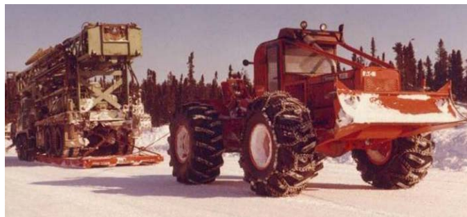
Above – An IWS drilling rig in tow across a frozen lake in northern Saskatchewan, used to drill dewatering holes for a uranium mine.
