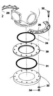
Tighten the bolts in the order shown in the illustration below. Tighten to 11 ft-lbs.
