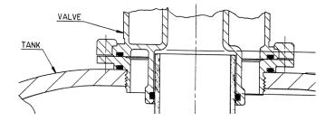
IMPORTANT: CES-2900E-300, Single CES-2900E-300-DP, CES-2900E-300-TP, and CES-2900-300-QP models only - distributor assembly (hub) should be positioned as close to the center of the mineral tank lower head as possible. Some mineral tanks have a rise in the center of the lower head that may require positioning the distributor assembly slightly off-center.
