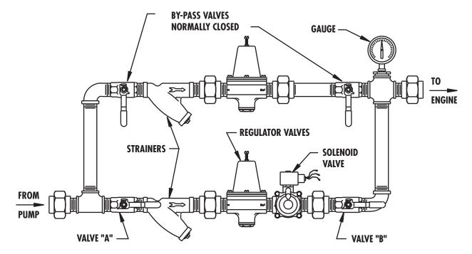
This instructional data explains the installation and operation of the cooling system for UL listed, FM approved Fire Pump engines equipped with heat exchangers.
