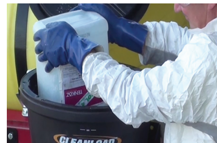
ProClean II Push Valve bottle rinse allows operator to triple rinse chemical containers on-site for legal disposal.
