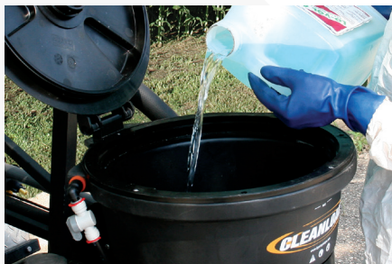
Educts 7 gallons (26.5 L) of liquid in 10 seconds and a 51 pound (23.1 kg) bag of AMS in 30 seconds.
