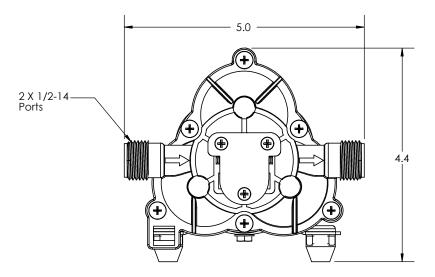
Installation Drawing 49 Wiring Removed For Clarity
