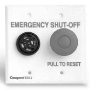
Select a convenient location to mount the ESO-2 Emergency Shut-Off Switch. Provide a double-gang electrical box. The electrical box must be rated for outdoor use if Emergency Shut-Off is located outside.
