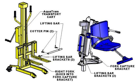
The AquaTRAM<sup>®</sup> Access Lift Transport Cart comes with a LIFTING BAR and two COTTER PINS, as shown above. The LIFTING BAR goes through the LIFTING BAR BRACKETS on the cart and the lift, and the COTTER PINS hold the bar in place. The right fork of the cart will also slide into the FORK CAPTURE BRACKET to keep the lift from tilting on the Transport Cart.
