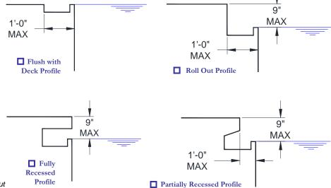
Caution: The AquaTram lift is not designed for pool profiles with curbs, walls or parapets. However, it <u>may</u> be able to clear very small curbs (up to 6" wide x 4" high) depending on curb location relative to the pool wall. Please do not order the AquaTRAM for use on a pool with even a small curb without confirmation of clearance from Pentair Applications Assistance: 1-800-831-7133
