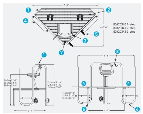
**1** The lifeguard station shall be a Griff's Vision Guard Station, no known equal. It shall have a triangular shape with the longer side facing front and completely open for unobstructed sight-lines and egress. Access shall be provided on each shorter side to facilitate lifeguard shift changes with uninterrupted coverage. The station shall provide for three lifeguard positions (two standing and one sitting) to facilitate the Griff's 5-Minute Scanning Strategy.
