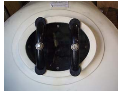
Correct yoke orientation
