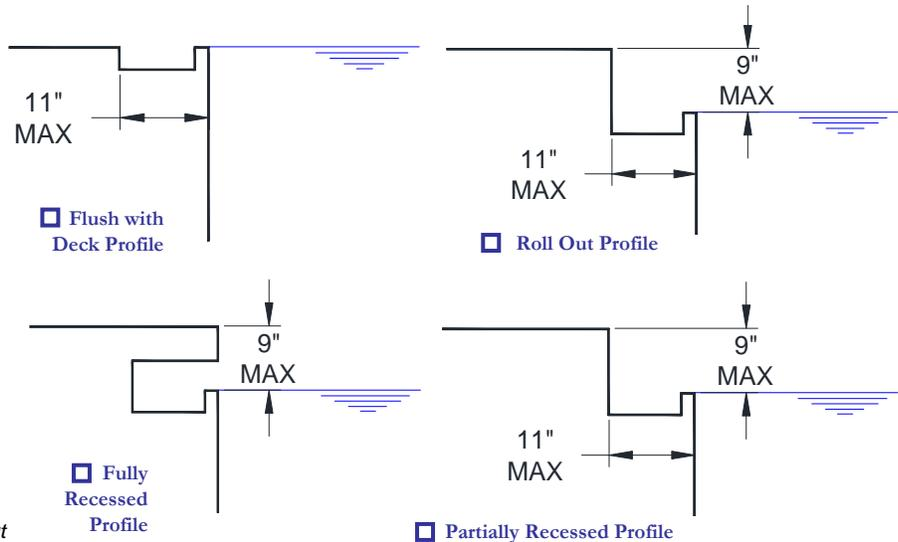
**Caution:** The AquaTram LT lift is not designed for pool profiles with curbs, walls or parapets. However, it may be able to clear very small curbs (up to 6" wide x 4" high) depending on curb location relative to the pool wall. Please do not order the AquaTRAM LT for use on a pool with even a small curb without confirmation of clearance from Pentair Applications Assistance: 1-800-831-7133
