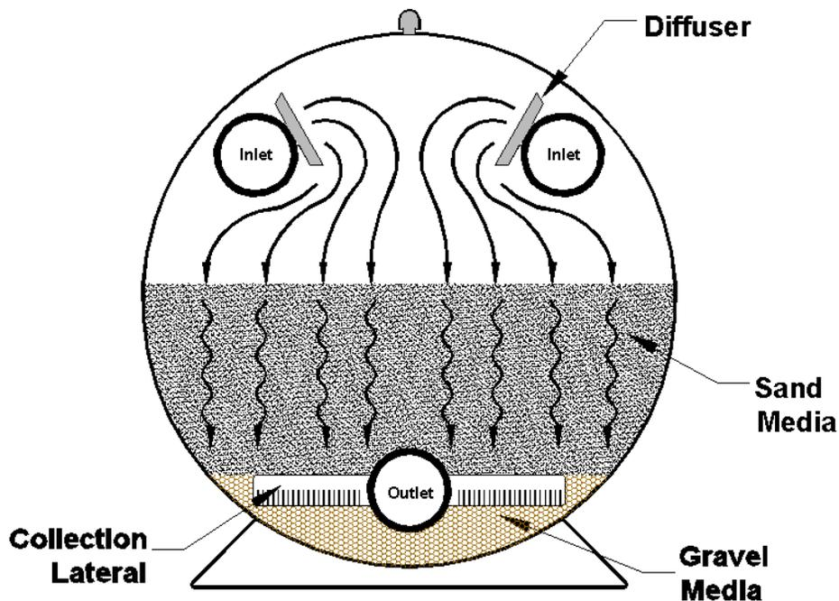
Tank Cross Section During Normal Filtration
