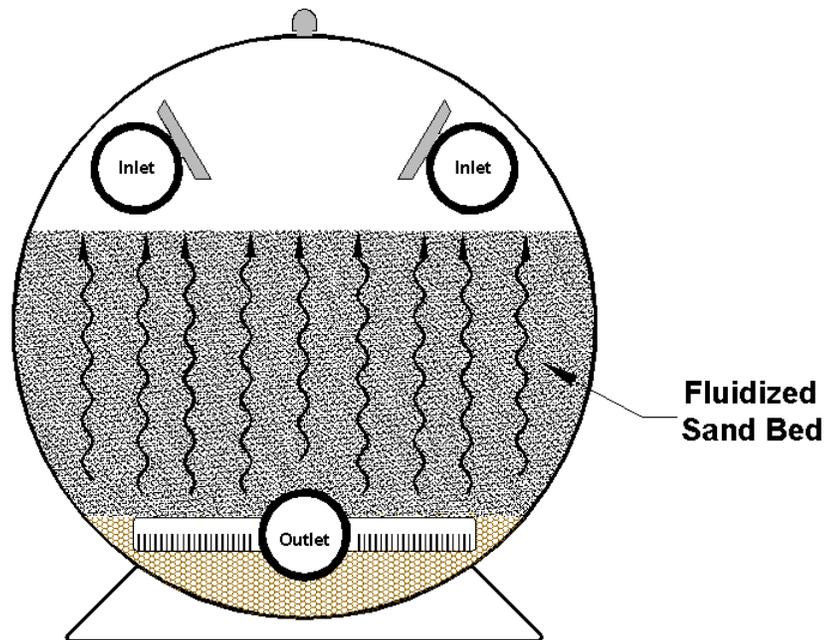
Tank Cross Section During Backwash Mode
