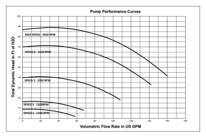
NOTE: The chart above demonstrates performance rates at factory preset speeds of 3450 RPM, 3110 RPM, 2350 RPM, 1500 RPM and 1100 RPM.
