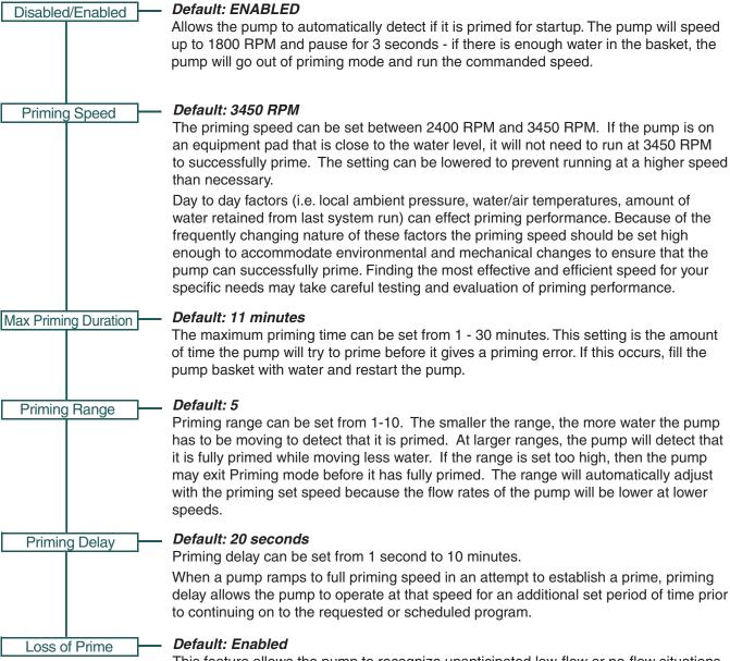
This feature allows the pump to recognize unanticipated low-flow or no-flow situations while running a program.
