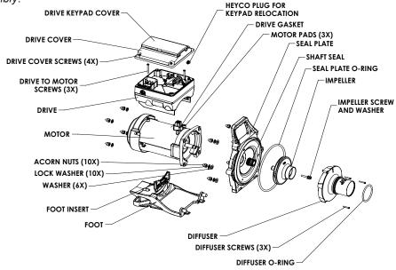
**Motor Assembly Breakdown**
