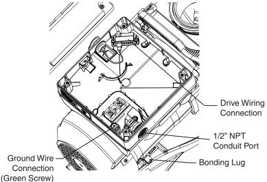
**Field Wiring Compartment**
