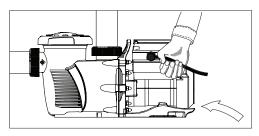
4. Reinstall the RS-485 communication cable.
