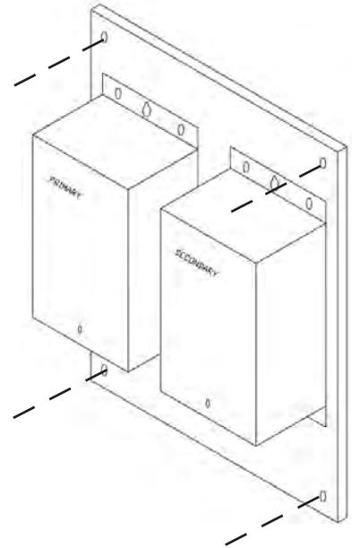
Mount power centers to wall using four (4) screws
