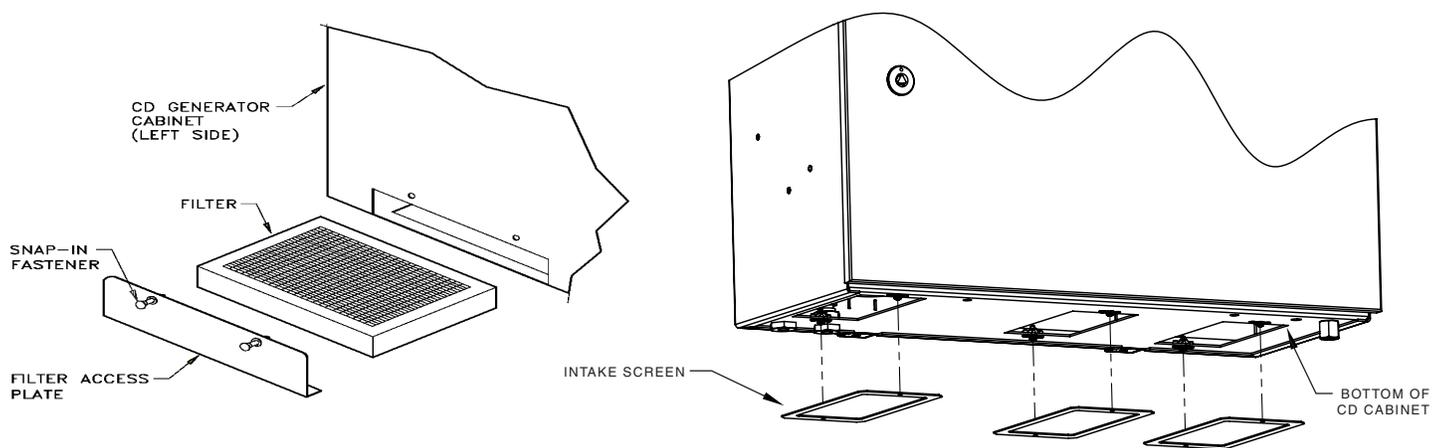
**Figure 5: Filter or Intake Screen Removal for Cleaning**
