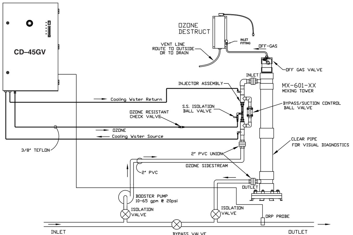
**Figure 2: Plumbing Schematic - Example of Swimming Pool Application**
