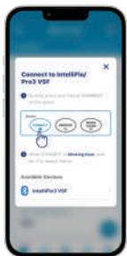
Press **Connect** at the pump. When the Connect button blinks blue, press **Continue** on the phone screen.
