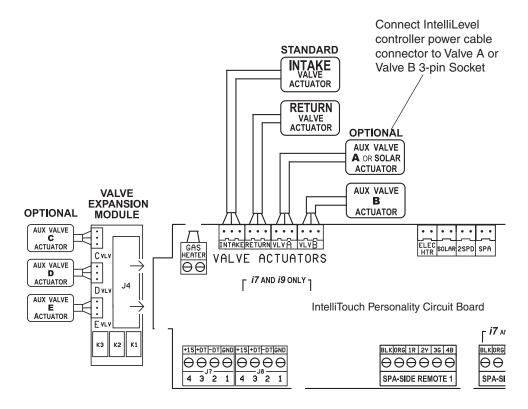
IntelliTouch Control System Circuit Board
