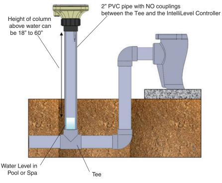
Main Drain Installation Diagram
