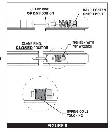
Note: Check the spring coils at least once a month to ensure proper tension. If spring coils do not touch then shut off pump and relieve pressure and tighten the nut and tap filter clamp until the coils touch.
