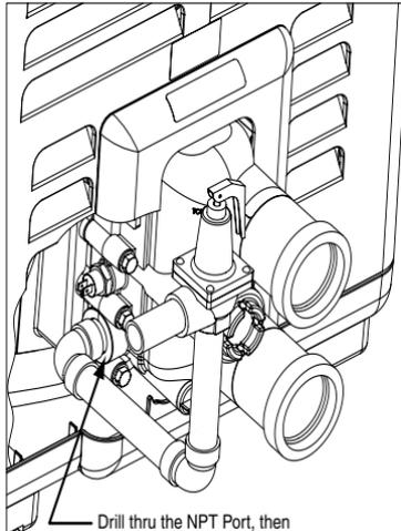
Drill thru the NPT Port, then use a 19 mm Brass Nipple and Elbow (user supplied) for a PRV Installation.
