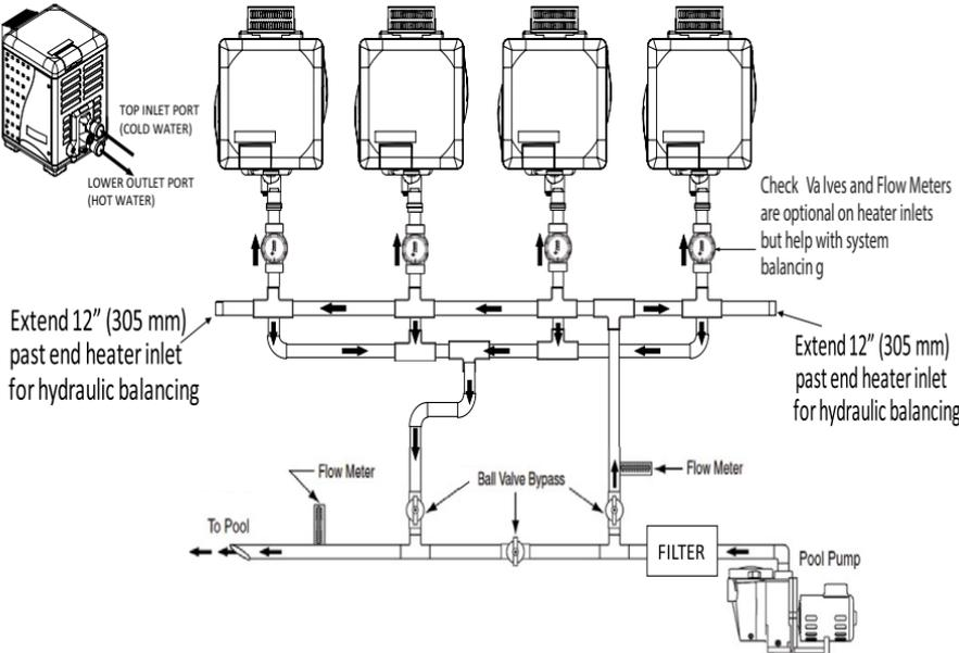
Figure 8. Four MasterTemp Heaters Plumbing Hydraulic Diagram
