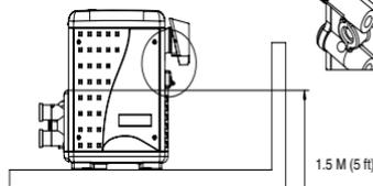
Turn star wheel **counterclockwise** to lower pressure set point if pressure switch is more than 1.5 M (5 ft) above water level
