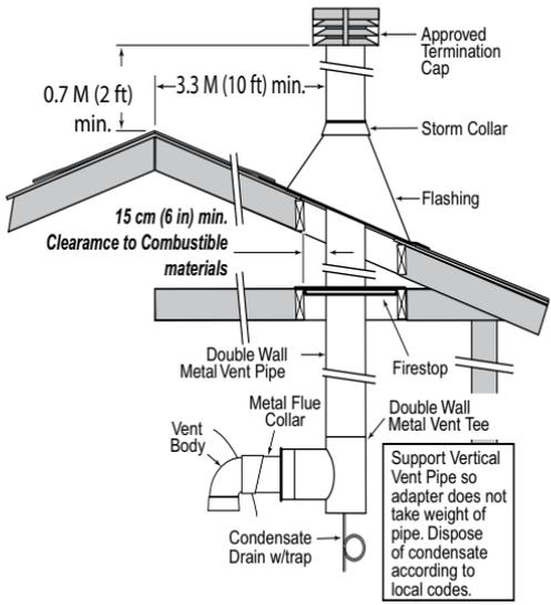
Figure 20. – Typical Metal Vent Pipe Installation (Vertical Venting)
