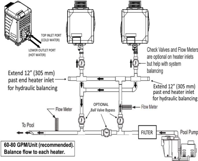
Figure 7. Two MasterTemp Heaters Plumbing Hydraulic Diagram
