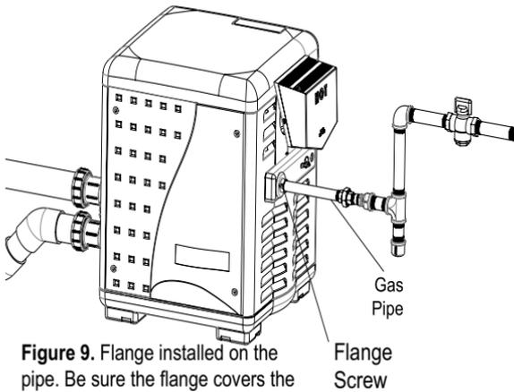
**Figure 9.** Flange installed on the pipe. Be sure the flange covers the circular opening in the heater panel.
