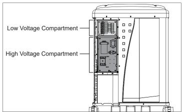
3. To access the Low Voltage Compartment, remove the four *Screws (1)* securing the Control Panel and allow it to swing downwards.
