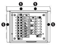
4. To access the High Voltage Compartment, remove the six *Screws (2)* securing the High Voltage Compartment Cover and place cover aside.
