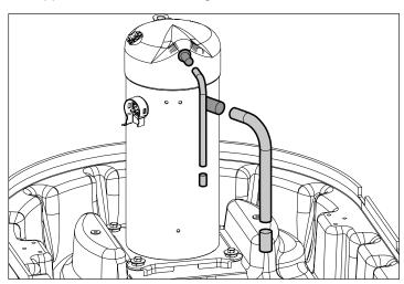
b. Cut the copper tubes to length. Clean and deburr the cut ends of the tubes.
