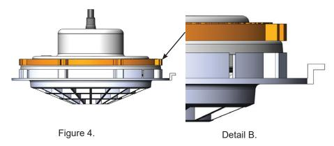
5. Insert one Truss head screw (11) into each of the 'U' shaped grooves on the clamp ring as shown in Figure 4.
