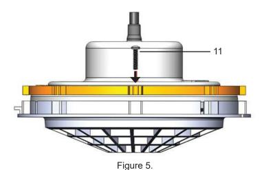
6. Hand tighten all eight screws ensuring all screw heads are flush with the top of the clamp ring. Follow the pattern in consecutive order starting from #1 and ending on #8 shown below in Figure 6. BE CAREFUL NOT TO CROSS THREAD THE SCREWS.
