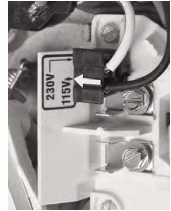
Figure 5B Voltage Change Plug Set for 115 Volts.
