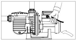
4. Reinstall the RS-485 communication cable.
