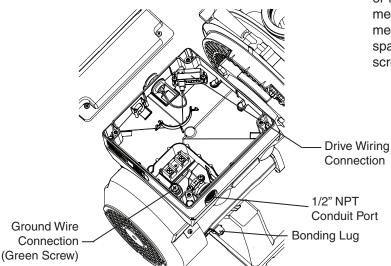
**Note:** When the pump is started and stopped by removing power with a relay or timer, a two-pole device should be used to apply and remove power to both POWER LINE TERMINALS.
