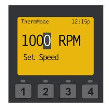
**Setting the Thermal Mode Pump Speed**
