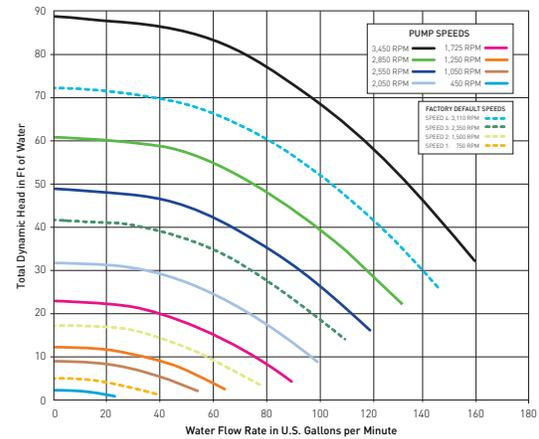
NOTE: The charts above demonstrate performance rates at factory preset speeds of 750 RPM, 1,500 RPM, 2,350 RPM and 3,110 RPM. However, flow rates can also be custom programmed between the ranges of 400 RPM and 3450 RPM.
