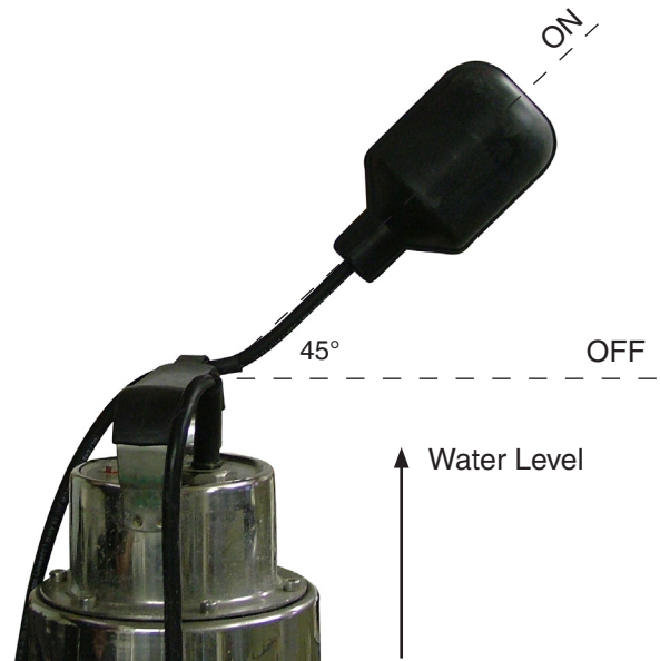
Float switch turns the pump on as it reaches approx. a 45° angle.
