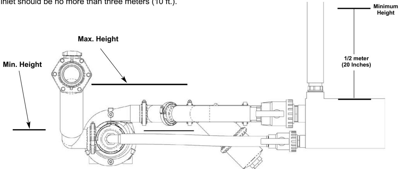
Mount self-priming adaptor in a location within 3 meters (10 ft.) of the pump inlet. The self-priming adaptor chamber is rated as a low pressure tank and is not designed to accept pressures over 3 Bar (45 PSI). System should be plumbed to protect from over-pressurization.
