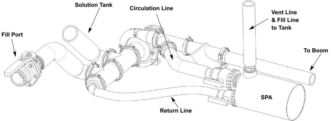
Manifold systems will function well with SPA. It is important to direct the return line from the SPA to the pump inlet in a manner as to jet the flow into the pump impeller to ensure good priming performance and stability. Use of Y fittings at the inlet of the pump will aid in accomplishing a positive
