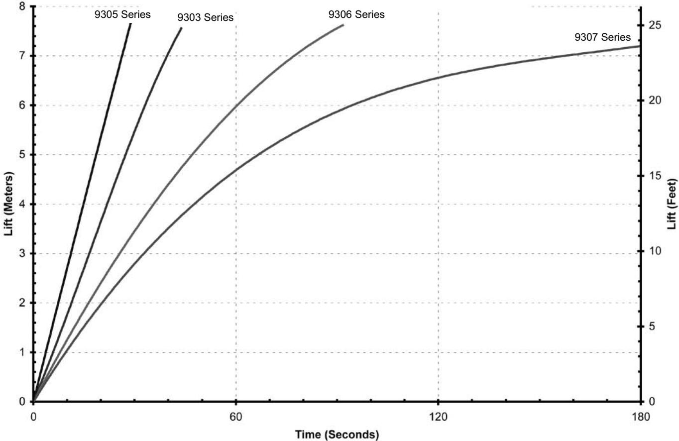
Priming rates are dependent on optimal plumbing systems, length and size of inlet hose, and rotational speed of pump impeller. Actual rates may vary depending on system configuration.
