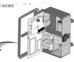
Wiring AC Power from IntelliChlor (SCG) and IntelliFlo<sup>®</sup> pump to IntelliTouch<sup>®</sup>, EasyTouch<sup>®</sup> and SunTouch<sup>®</sup> Control System (see page 27 for diagram)
