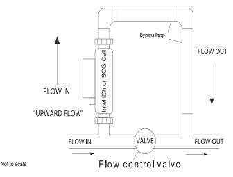
IntelliChlor SCG System Loop Plumbing Diagram
