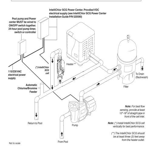
IntelliChlor SCG System Schematic Diagram
