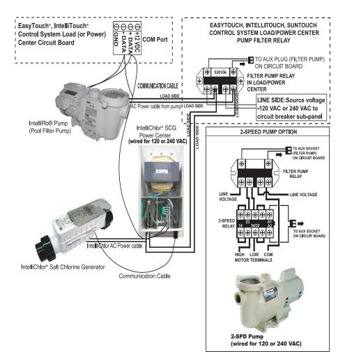
Wiring IntelliChlor® SCG AC Power Cord to Automation Control System Filter Pump Relay
