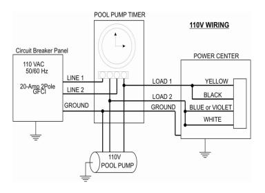
115 VAC Basic System Wiring with Pool Pump Timer
