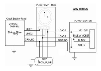
220 VAC Basic System Wiring with Pool Pump Timer
