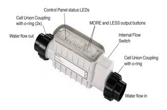
IntelliChlor® Salt Chlorine Generator (SCG) Cell
