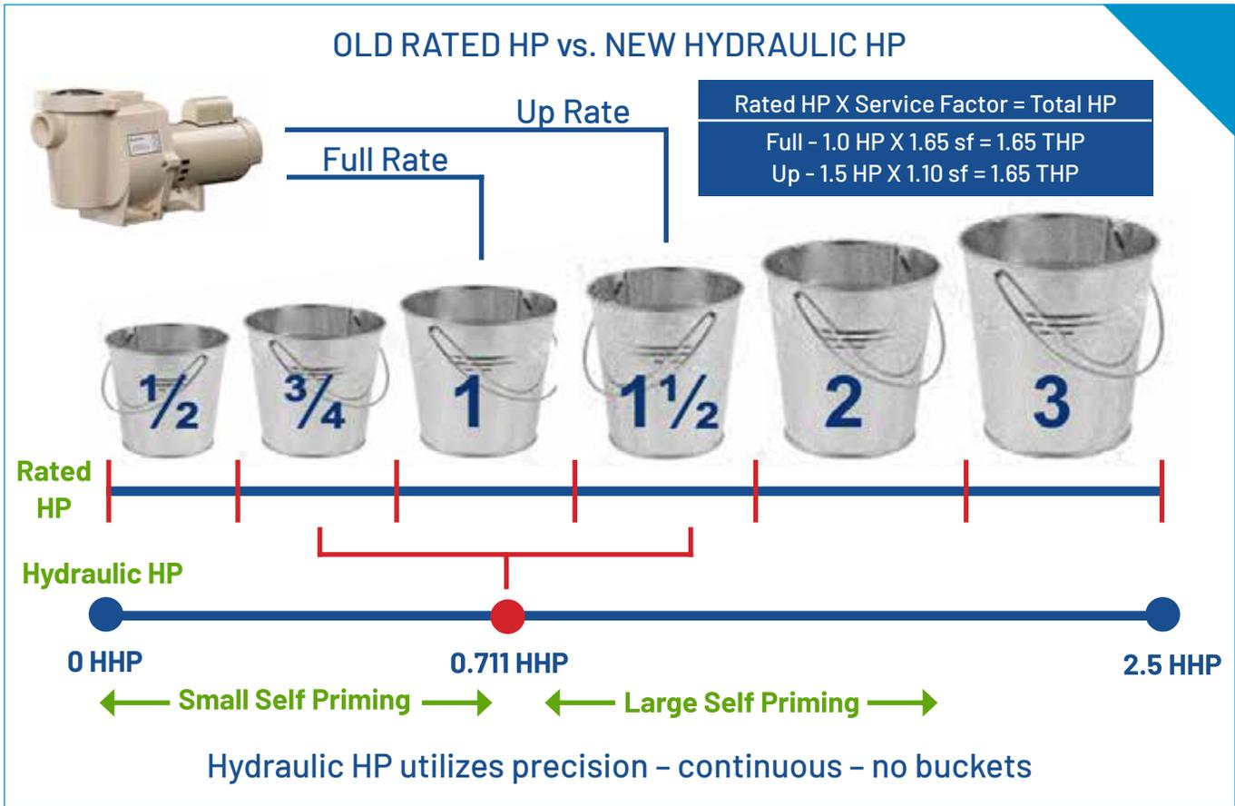
The old method of identifying pump sizes was rated horsepower. Going forward, the DOE regulation will require HHP ratings, which are more useful because HHP is a better indicator of a pump's performance.
