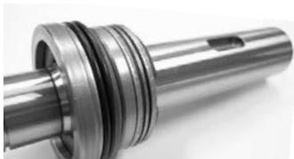
10. Do not press, but place the shaft sub-assembly into the motor body with threaded end of shaft up. Lubricate the two o-rings with hydraulic or mineral oil before assembling.
