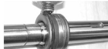
8. Identify new type front spacer provided in kit used only on old type motors. Discard old front spacer from the disassembly. (New type front spacer looks like a thick washer with a counter bore on one side, approx .164 inch thick).
