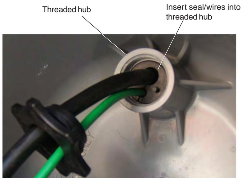
9. Slide the seal cap into the niche threaded hub. Carefully position and align the cap with the threaded hub. Hand tighten the cap clockwise two or three turns.
