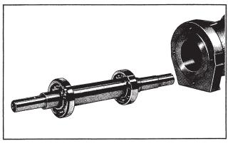
1. Shaft assembly removed
