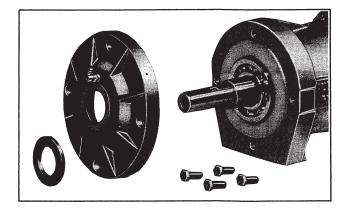
H. Bearing cap and slinger removed
