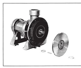
E. 1st stage impeller, key and gaskets removed
