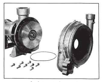
D. Casing and gasket removed
