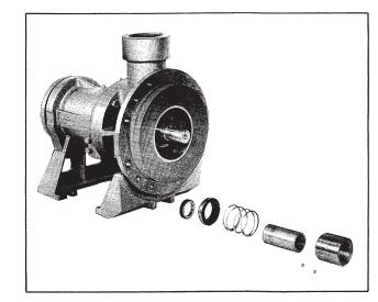
F. Mechanical seal and sleeves removed
