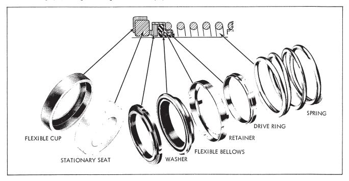
Figure 1. Mechanical Seal (Optional)
