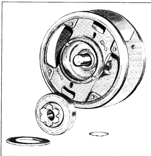
C. Slinger, bearing collar, bearing and retaining ring removed.
