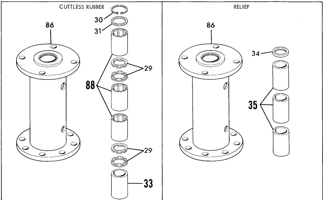
Figure 1. Model 641-642 Exploded View (Sheet 3 of 3)
