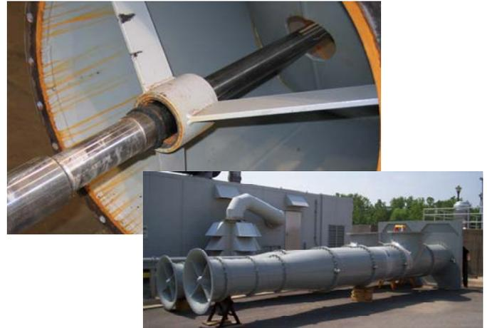
*The upper rubber lineshaft bearing burned up on the sleeve, fell out of its retainer and slid down the shaft.*
