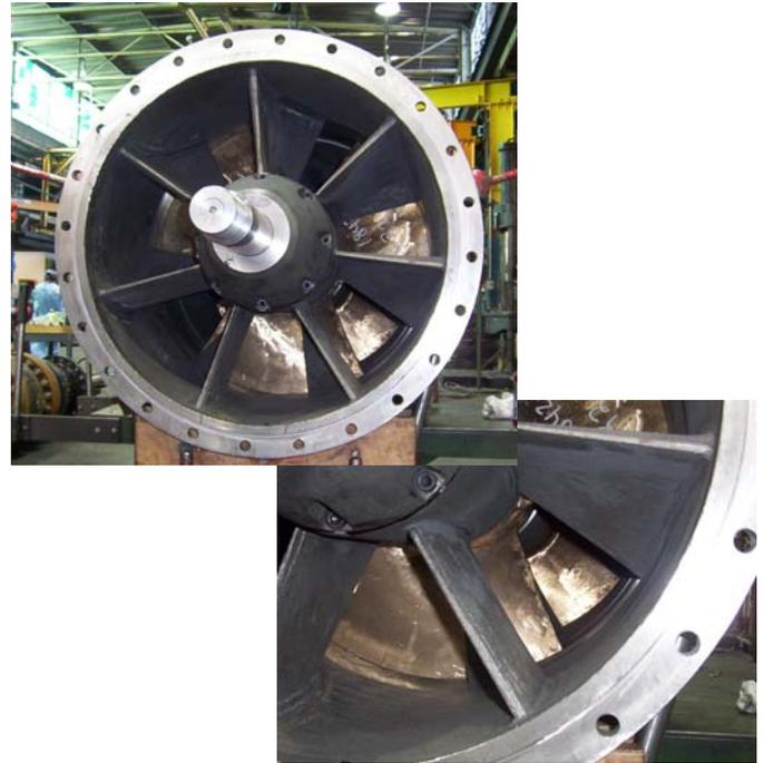
Discharge of the 500 HP two-stage 30P bowl assembly can be seen above. Once each bowl is complete, it is given a performance test. Then the rest of the pump including column, shafting, discharge elbow, and pedestal is assembled, painted, and ready for shipment. Pictured below are two-stage 24P and 30P bowl assemblies prior to testing.
