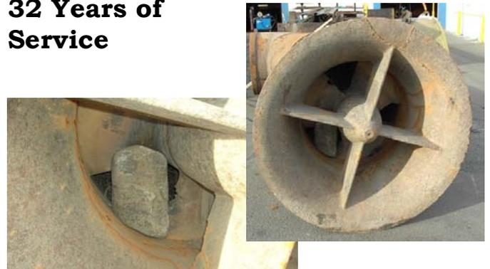
This Verti-Line 36P propeller pump was first installed in 1974 for Manitoba Water Stewardship in The Pas, Manitoba. Driven by a diesel engine via right angle gear, the pump operated until early 2006 when a rock was sucked into the impeller. Long time Verti-Line distributor National Process Equipment (formerly Wilron Equipment) in Canada pulled the pump for repair. Pictures courtesy of Mike McDonald at NPE.
