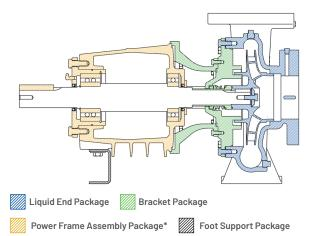
\*Power frame assembly package includes shaft & foot support package by default.
