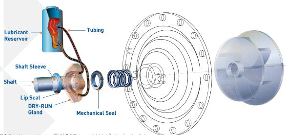
The DRY-RUN Gland incorporates two (2) 1/4" NPT tangential inlet (bottom) and outlet (top) ports. The rotating shaft provides a pumping action inducing a continuous flow of lubricant from the reservoir to the gland and back through the bottom and top ports. The "Turbulator" channels fluid to outlet port, limiting recirculation and
