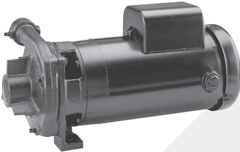
The Type C Pump is a compact, horizontal, single stage, centrifugal pump close-coupled to an electric motor. The removal of readily accessible bolts (back pull-out construction), permits the removal of the pumping element, exposing the impeller and seal for inspection, without disturbing the piping.
