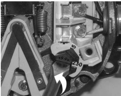
Figure 12 - Changing the Voltage Setting
