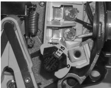
Figure 13 - Motor Set for 115 Volt Operation
