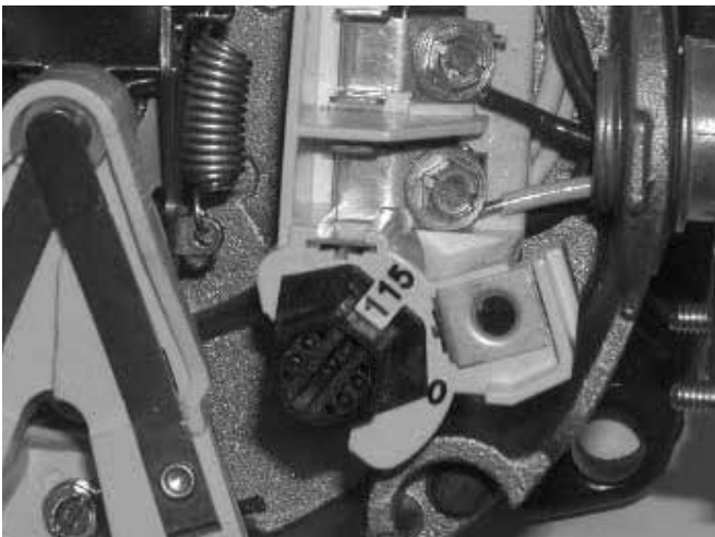
Figure 6: Motor Set for 115 Volt Operation.
