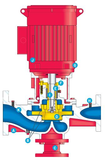
NOTE: Front case wearing rings are standard on all size pumps. Rear case rings are standard on all sizes except the 2x2x9C. The 2x2x9C does not require a wear ring.
