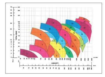
Shown are performance curves according to the bowl sizes and types in the Vertical Turbine line ranging from 1200–3600 RPM.
