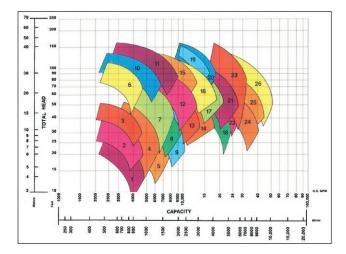
Shown are performance curves according to the bowl sizes and types in the Vertical Turbine line ranging from 440–1800 RPM.
