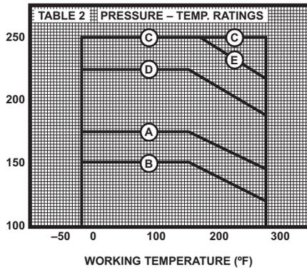
EXAMPLE: A model 1900 pump with a bronze casing has been selected for operating at a case working pressure of 240 psig at 150°F. Enter Table 2 at 150°F and read upward to 240 psig. It is determined that the selection is within the recommended maximum case working pressure area for 300 psi flanges and is therefore acceptable. Note that the example exceeds the maximum case working pressure unit if the material selected would have been 125 psi flanged cast iron or 150 psi flanged bronze.
