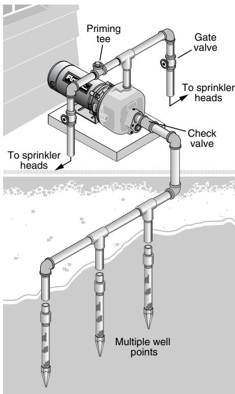
**Figure 2: Driven Point Installation,
