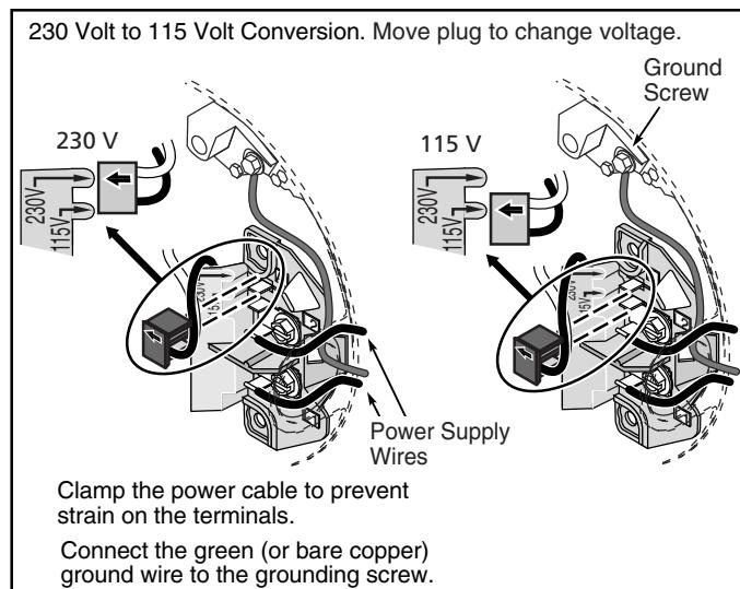
Connect power supply wires to L1 and L2. For 3-phase motors, or if motor does not match these pictures, follow the connection diagram on the motor nameplate.
