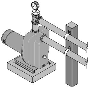
Figure 9 – Independently Support All Piping Attached to Pump
