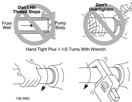
Figure 11 – Don't overtighten
