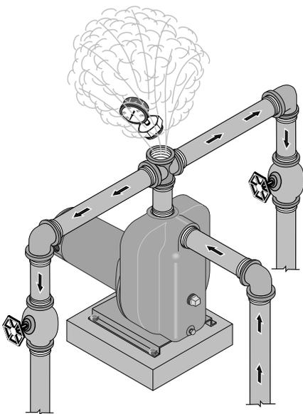
**Figure 15 – Do Not Run Pump with Discharge Shut-off**
