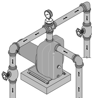
Figure 7 - Refoulement multiple
