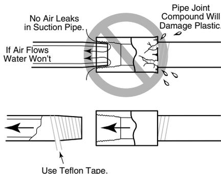
**Figure 4 – Suction Pipe Must Not Leak**
