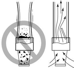
**Figure 2 – Foot Valve Must Work Freely**
