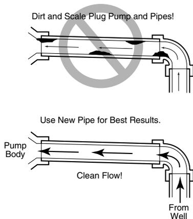
**Figure 1 – No Dirt or Scale in Suction Pipe**
