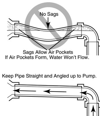
**Figure 3 – No Air Pockets in Suction Pipe**
