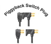
The piggyback design allows for simple conversion to manual operation by simply removing the switch plug and inserting the motor plug directly into the electrical outlet. This feature provides an easy way of periodically cycling the pump to ensure it is operating properly.
