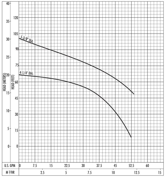
The curves reflect maximum performance characteristics without exceeding full load (Nameplate) horsepower. All pumps have a service factor of 1.2. Operation is recommended in the bounded area with operational point within the curve limit. Performance curves are based on actual tests with clear water at 70° F. and 1280 feet site elevation.
