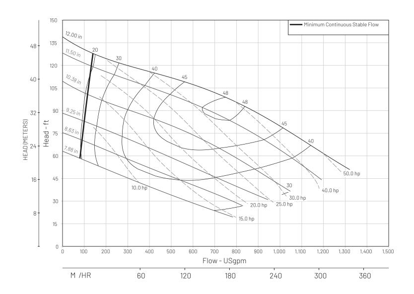
The curves reflect maximum performance characteristics without exceeding full load (Nameplate) horsepower. All pumps have a service factor of 1.2. Operation is recommended in the bounded area with operational point within the curve limit. Performance curves are based on actual tests with clear water at 70° F. and 1280 feet site elevation.
